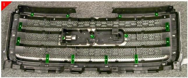
First locate the main outer trim ring and the mesh center. Lay trim ring on a protective work surface, next place the mesh and align so that the mesh clears the mounting studs. Next place trim ring and mesh into stock grille shell opening and center. Place the supplied brackets in place and secure with the supplied 10-24 nyloc nuts. Check alignment before final tightening of the nuts.
