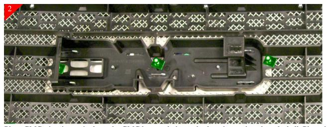
Place GMC trim ring so it clears the GMC logo and the studs clear the mesh and stock shell. Place the supplied small square brackets in place and secure with the supplied 10-24 nyloc nuts. Check alignment before final tightening of the nuts.
