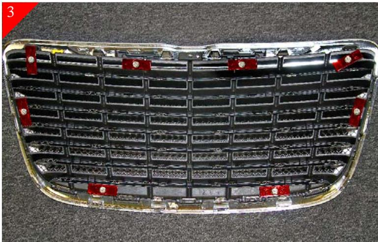
3 With ring and mesh together place stock grille shell on top of trim ring and mesh and center. The mounting studs pass through the stock grille shell and then place supplied (shown in RED) brackets and secure with 10-32 nyloc nuts as shown above. Check alignment before fully securing in place.
