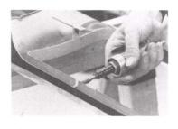
STEP 9 With a rotary tool or round file, grind notches into the rim 1/4" wide and approximately 5/8" deep, which the vertical bars will fit into.
