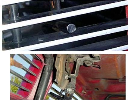
**Step 5 (1997-1998)** You will now need to install the hood release extension by clamping the extension onto the secondary hood release with the rod pointing toward the front. Mark and drill 1/4" holes and bolt in place. The extension will protrude just beyond the billet grille. (1997-1998) Remount factory shell with billet inserts onto truck. **For 1999 & later see step 6.**
