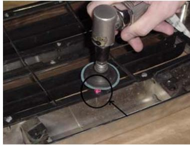
**Step 2** Using a grinder remove the plastic welds which hold the louvered section in place. This will allow you to remove all louvers.
