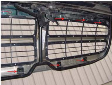
**Step 1** Remove factory grille shell from truck. Lay face down on padded surface to keep from damaging finish.
