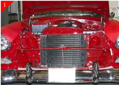
Start by removing the Trim ring around stock grille shell. You do not need to remove the Trim piece that's attached to the hood. Then remove the Stock grille by removing screws along the top & bottom of grille. There are 2 bolts in the left & right fender area that need to be removed in order for the center section to be removed.
