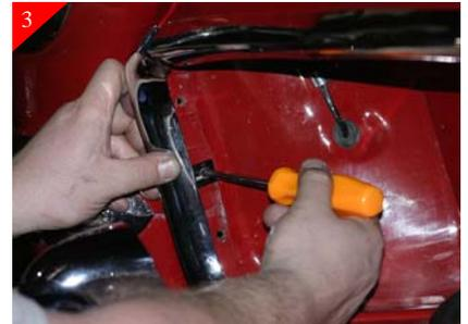
Next hold side trim piece up to vehicle with the hood shut and align trim piece as shown. Then using a scribe or sharpie mark the locations of the brackets to be drilled. Then using a 9/32" drill, drill in the just marked locations for mounting the trim. Using the supplied 1/4-20 Soc head bolt and 1/4-20 nyloc safety nut attach brackets to vehicle. Do not tighten brackets at this point, leave loose.
