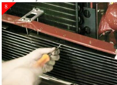
Place the supplied U-clips on both sides of the supplied Top billet grille brackets. Then attach brackets to billet grille using the supplied #8 x 5/8" Phil pan head screws. It is not necessary for the billet grille to be placed into opening for attaching top billet grille brackets.
