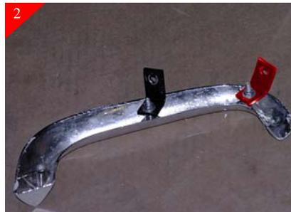
Next attach the supplied brackets to the left & right Trim pieces as shown. You will be using the stock trim posts & stock nuts to attach the brackets. NOTE: The bracket shown in RED is left and right specific.
