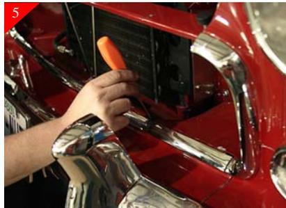
With the bottom trim piece in place you will need to mark the locations of the brackets. Then drill a 9/32" hole in each of the marked locations. Then attach bottom trim by using the supplied 1/4-20 Soc head bolt & 1/4-20 nyloc safety nut.
