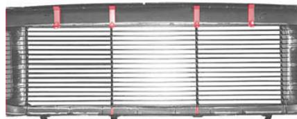
**STEP 4** Attach upper brackets to billet grille using 1/4-20 nuts & bolts. Lay grille shell face down and center billet grille in opening. Mark location of rods as shown above. Drill an 1/8" hole in each marked locations. Now attach grille, buy using self tapping screw in each of the drilled locations. Snap grille shell with billet grille into place. Mark and drill an 1/8" hole in each bracket location. Attach upper with 3/4" self tapping screw, in each drilled location.
