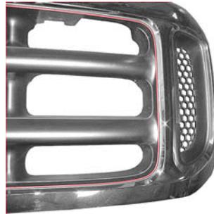
**STEP 2** Place grille on protective work surface such as a work bench with a blanket. Then tape off the chrome portion of the grille with masking tape so you don't scratch the face of the grille shell. Notice that there is a molded line in the shell about 1/8" inside the chrome as shown above.
