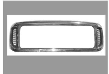
**STEP 3** Cut out the grey plastic center of the grille shell being careful to follow the small grey molded line described in step 2. After cutting the center out use a file to smooth out the edges. Again being careful to follow the grey molded line. NOTE: If installing center only skip step 4. You don't need to cut out the left and right pockets.
