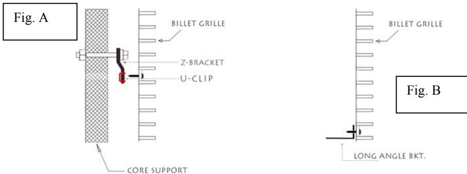
Step 3: Attach the (2) Long Angle Brackets to the 2-center tabs on bottom of billet grille as shown above (Fig. B).
