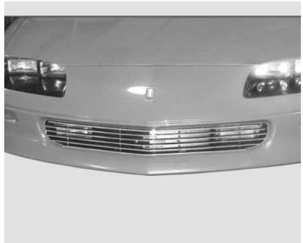
STEP 3 Attach grill using the supplied 4 - #10 x 1 1/4" as shown.
