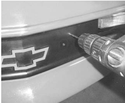
STEP 2 Drill 1/8" hole at each marked location.
