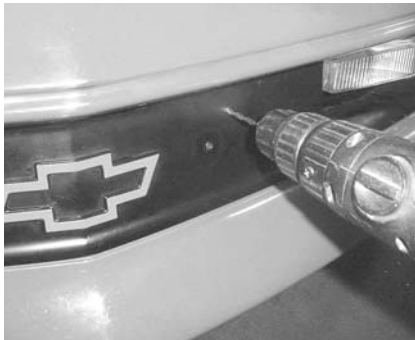
STEP 2 Drill 1/8" hole at each marked location.
