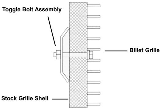
**1.** Center billet grille in opening. Using the supplied Toggle Bolts attach per illustration above.
