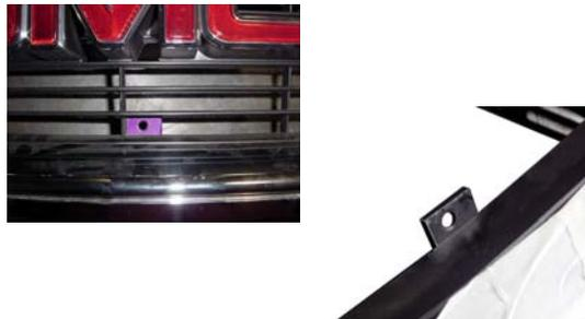
**STEP 5** Using a cut-off wheel or hacksaw, cut around the bottom mounting tab. **This mounting tab is necessary to retain the shell to the vehicle.**
