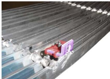
**STEP 8** Attach the long edge of the brackets to the billet grille using the supplied hardware as shown.
