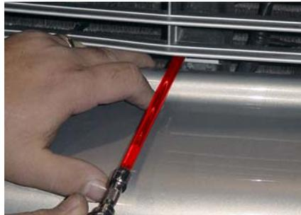
**STEP 2** Remove (1)-7mm screw from the bottom of the grille shell between the bumper and bottom bar of grille shell as shown above.
